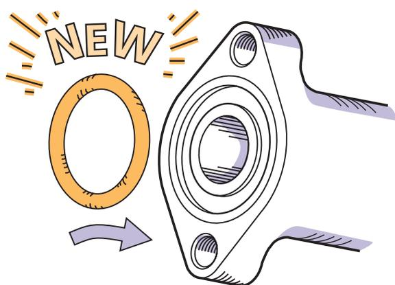
Pinched oil rings will cause oil leaks and lower oil pressure.
