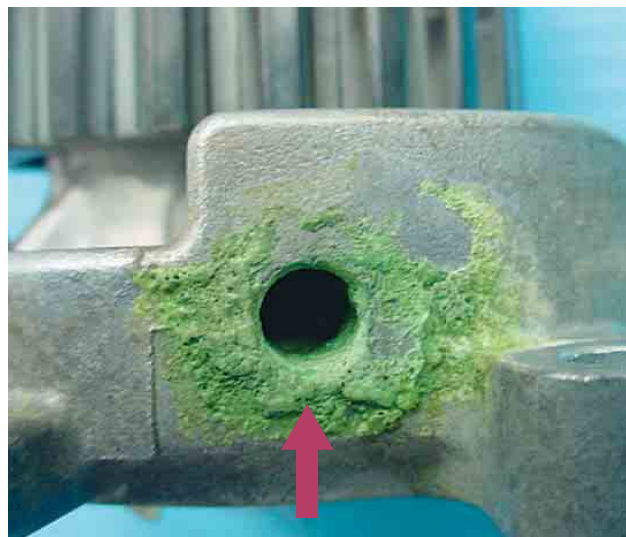
Damaged Large coolant bleed mark, dampness or dripping.
