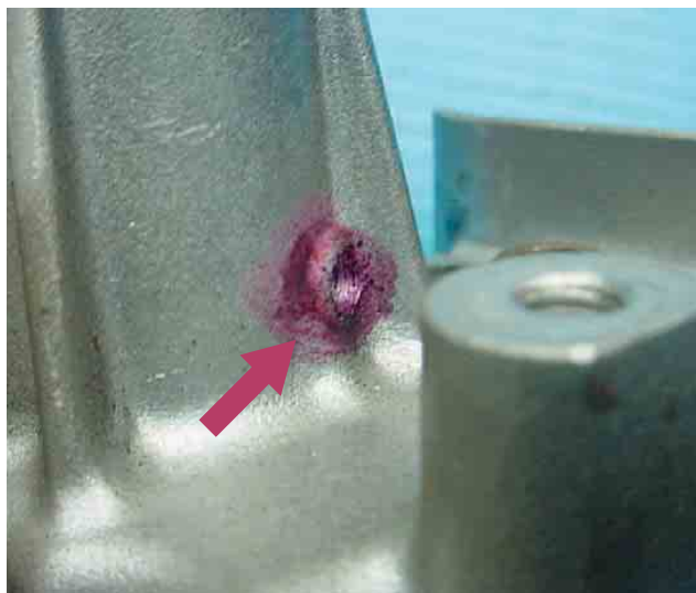
Normal Dried coolant residue.
