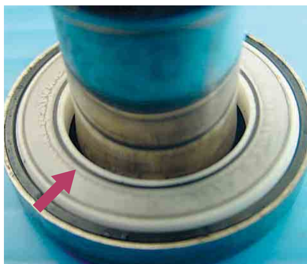
Damaged Accumulated sludge (Contaminated coolant).
