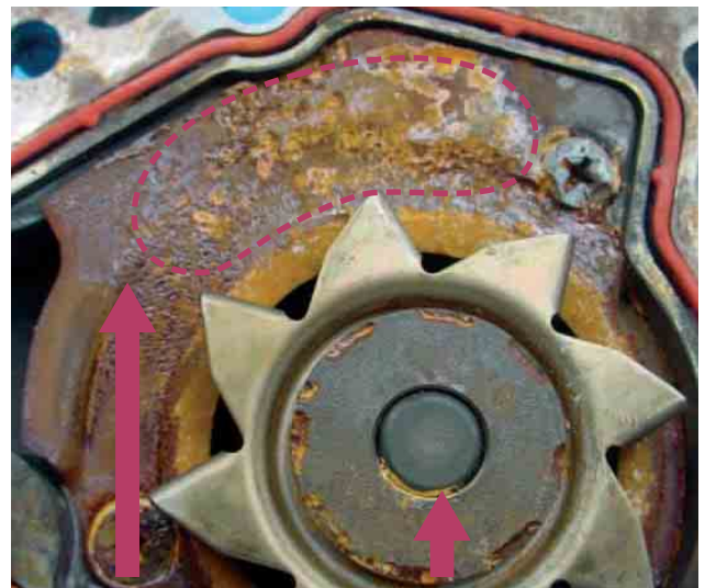
Cavitation Corrosion around crimp
