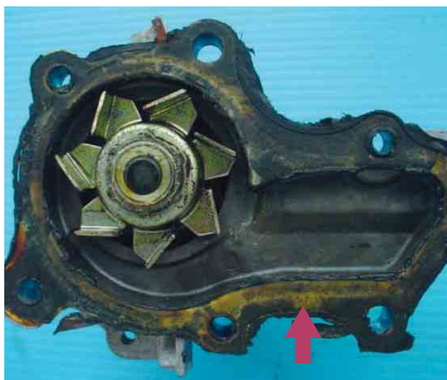
Insufficient accuracy on the mounting surface.
