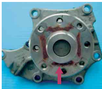
Flecking at the pulley seat
