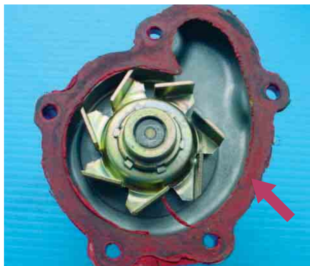
Gasket performance has degraded.
